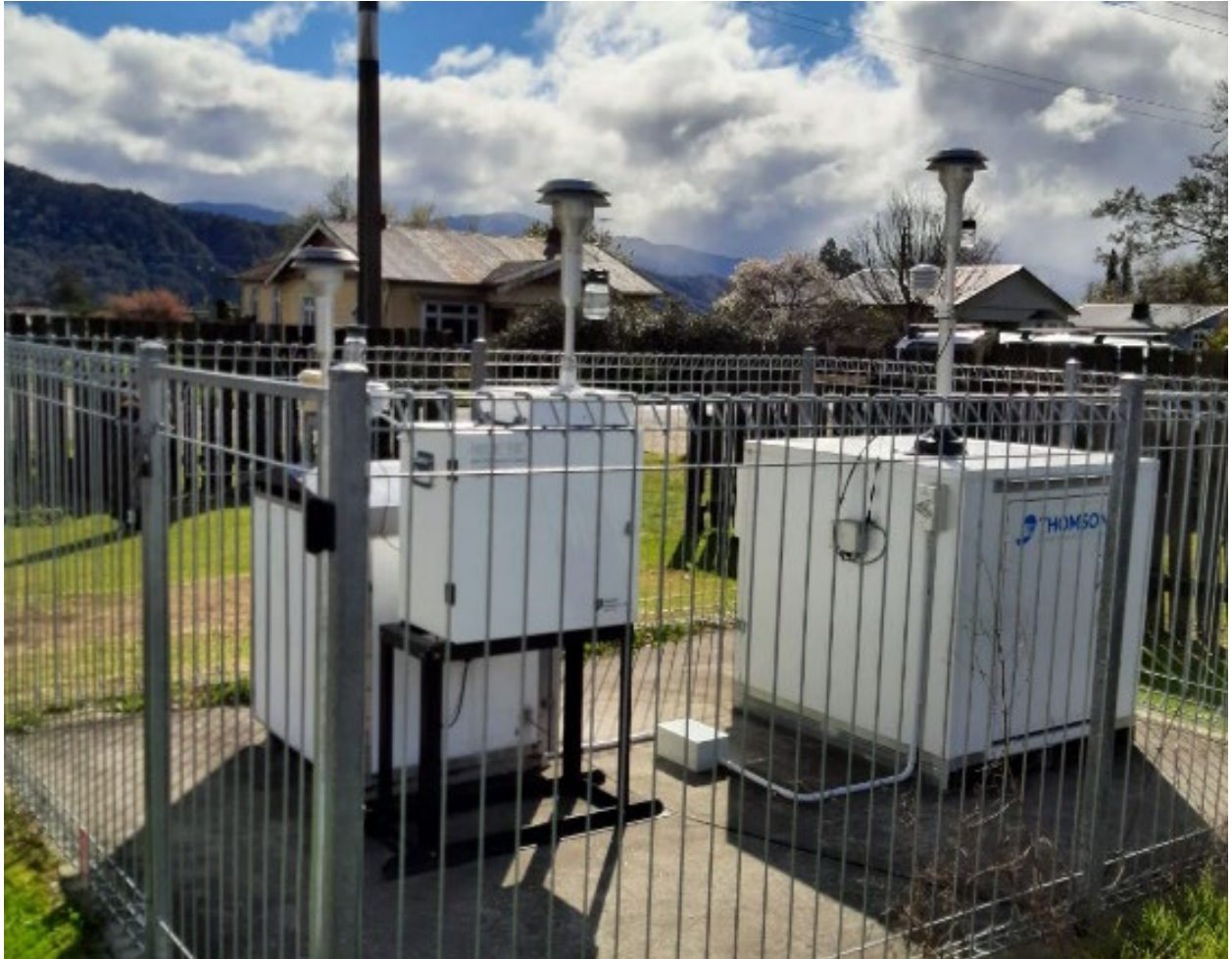
Figure 2. Reefton air quality monitoring instruments. From left to right; BAM, Partisol, and T640X.
